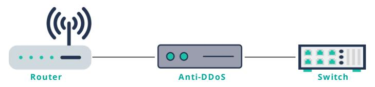
The On-Premise Anti-DDoS solution above is placed between the external router and the next hop - in this case a switch. As the Anti-DDoS solution is deployed inline in Transparent Layer 2 mode, the router assumes all packets it is receiving are coming from the switch and vise-versa. Hence, neither the router nor the switch is aware of the presence of another network device and assume they are directly connected to each other - making the Anti-DDoS device invisible.
